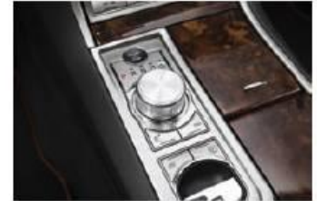
Figure 2.2 Trackerballs are used in some luxury cars to select functions such as radio, telephone, music and satnav
